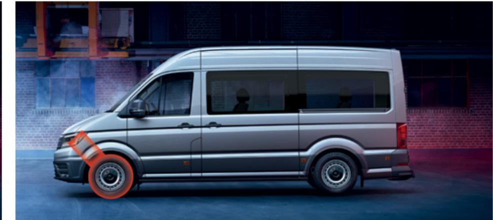
The Crafter Minibus comes standard with an 8-speed automatic with torque converter transmission, along with a 2.0L TDI410 bi-turbo (410Nm, 130kW) engine, of which both have been developed and calibrated especially for the Crafter's specific driving characteristics, providing great response even under load, also offering the highest performance and durability requirements.
