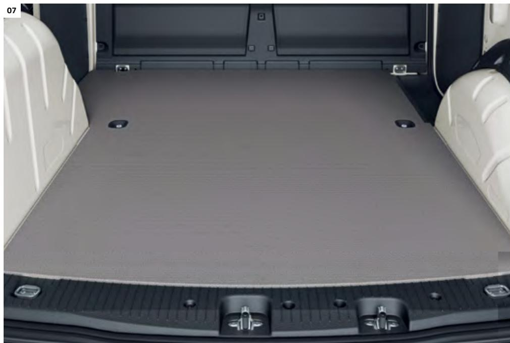
**07 Wooden floor.** Can easily cope with even hard blows. The particularly sturdy load area covering made of multi-bonded beech wood protects the vehicle floor and impresses with its water-resistant and non-slip surface. | C |
