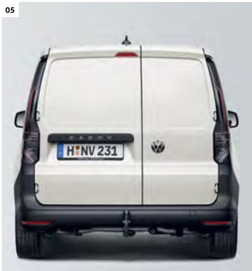
**05 Rear wing doors without windows.** The roof-high rear wing doors are split in the ratio  $\frac{2}{3}$  to  $\frac{1}{3}$  and have a maximum opening angle of around 180°. | C | CR |
