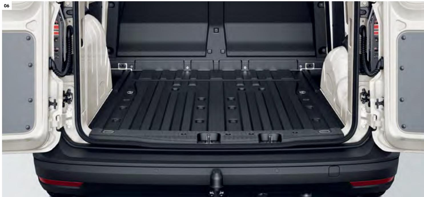
**06 Rubber floor covering.** Increases safety thanks to a non-slip surface. The robust rubber floor covering can be simply washed clean in the event of heavy soiling. | C |
